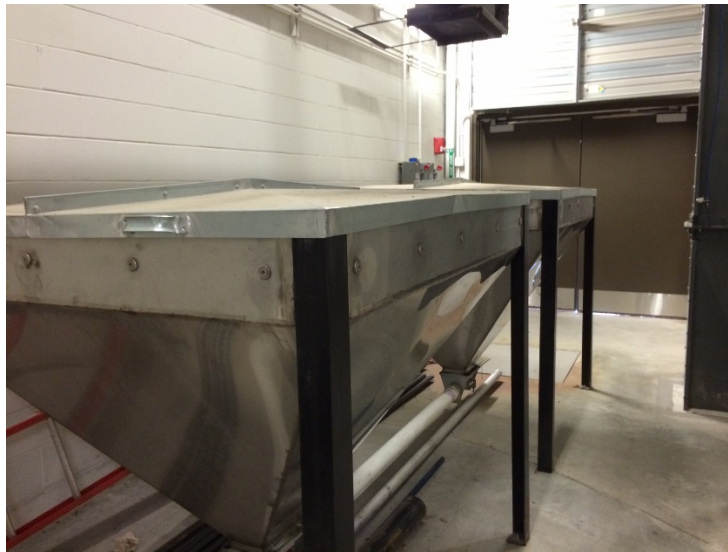
Figure 3.4: Secondary Fuel Bin
